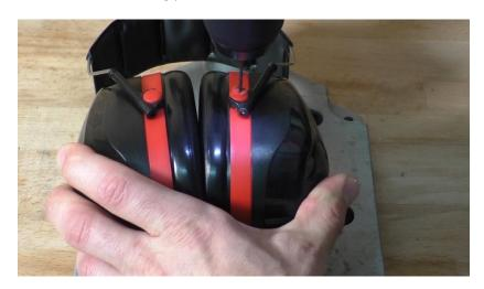
If the pin is made of plastic, take a metal drill, drill a shallow hole into the pin, but make sure **not to penetrate** the pin/housing. Take a screw, cut it to a suitable length using the saw or pliers, if necessary, and screw the magnet to the hearing protection.
